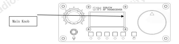
The five multi-function buttons at the bottom of the screen correspond to the displayed function menu.
