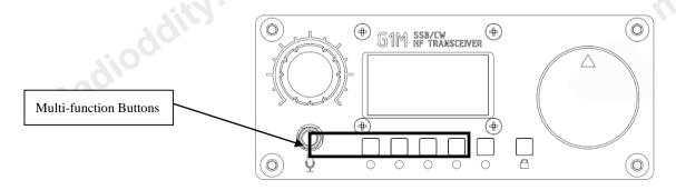
Momentarily press the "lock" button to switch the menu page. Hold press the "lock" button to lock the button operation.
