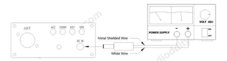
When the G1M uses an external power supply, in order to prevent external interference from entering the radio through the power line, please place a snap-on ferrite choke close to the DC plug. Loop the DC cord through the choke a few times.
